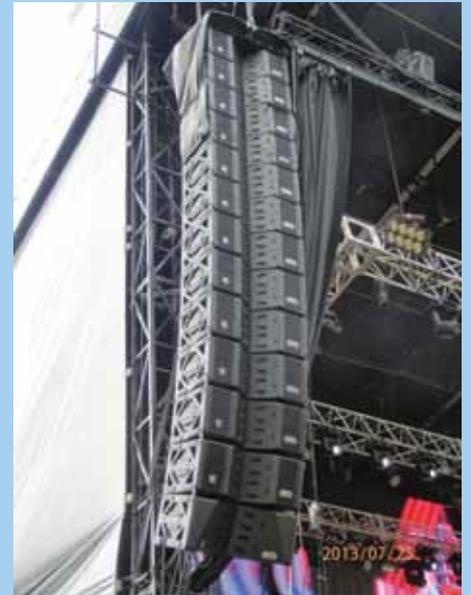
Featuring multiple stages, the 'White Stage' was equipped with an Outline large-format line-source rig: 24 GTO elements, 2 GTO-DF (Down-Fill) and 18 ground-installed DBS 18-2 subwoofers.
