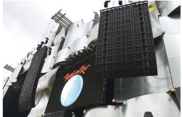
The main hang included 120 VerTec VT4889 and 84 VT4880A
