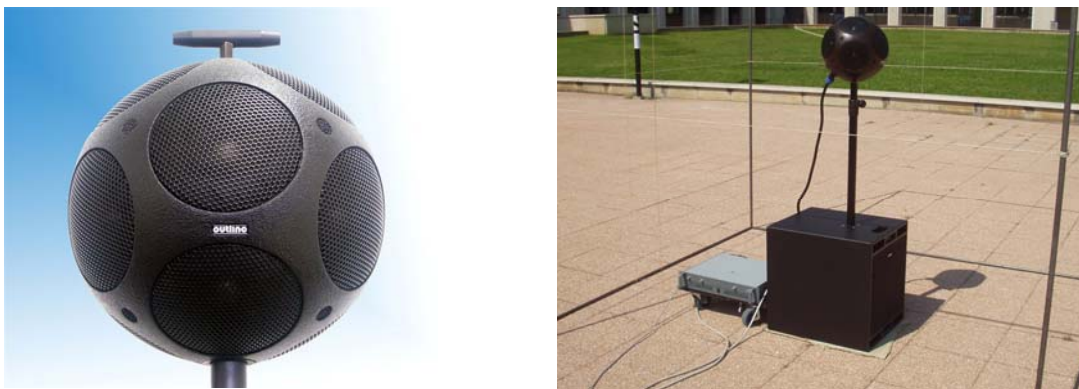
Figure 1: Close-up of the omnidirectional enclosure and a view of the complete system.
