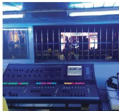
The 6,000-capacity theater's FOH setup includes an iLive-T112 control surface with an iDR-48 MixRack.
