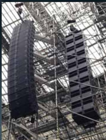
The STM Series is completely modular and is comprised of 4 elements – M46 main cabinet, M28 omnipurpose main or downfill cabinet, B112 bass cabinet and S118 subbass cabinet. There is total flexibility to configure a system that is suitable for audiences between 1000 and 100,000 although Nexo has received reports from events where the crowd was 200,000+. The rental company can use all 4 elements to create one of the most powerful line array systems currently
