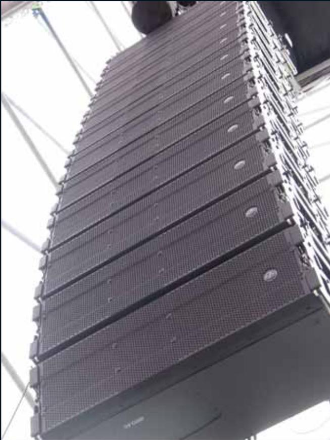
Aero 40A Advanced Line Array System is a 3-way powered line array system which incorporates connectivity for remote monitoring and control. The unique configuration of the Aero 40A employs a rear-loaded 12" transducer in a bass-horn configuration for low-end reproduction. The mid-range is handled by a new 8" transducer developed specifically for the Aero 40A. High frequency reproduction relies on two D.A.S. M-75N compression drivers attached to a new BPS-2912 waveguide.
