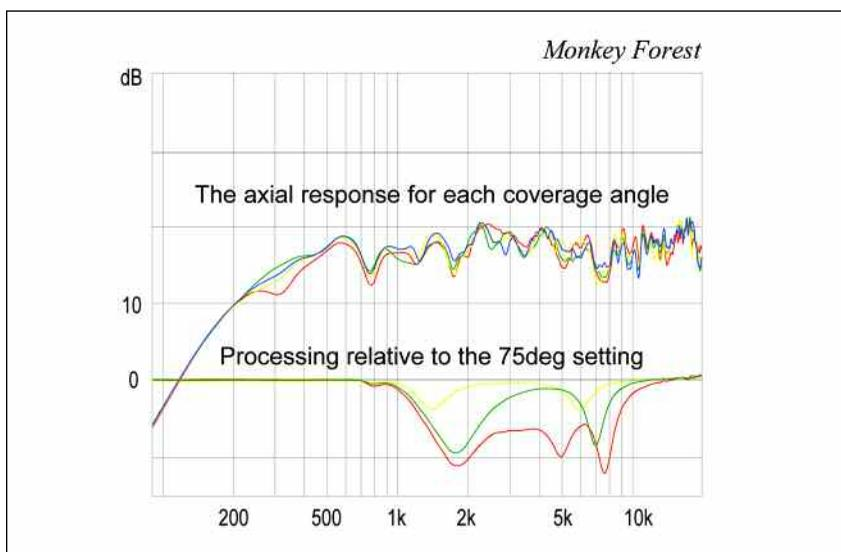
Figure 2 – The axial response for each sidewall and switch setting. I tested symmetrical configurations only.
