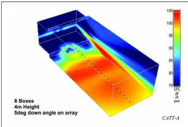
Figure 14 – Array 2 at 4m height.
