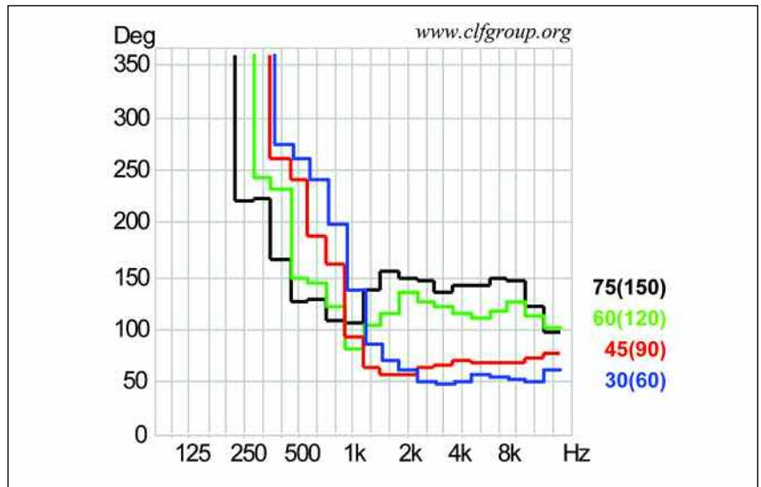
*Figure 4 – The horizontal beamwidth vs. frequency for each setting of the mechanical sidewalls (and processing switches) of a single MiniCOM.P.A.S.S.*
