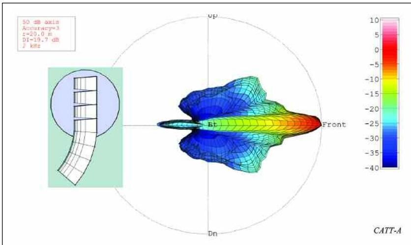
Figure 8 – 2 kHz balloon of the straight segment of Array1.
