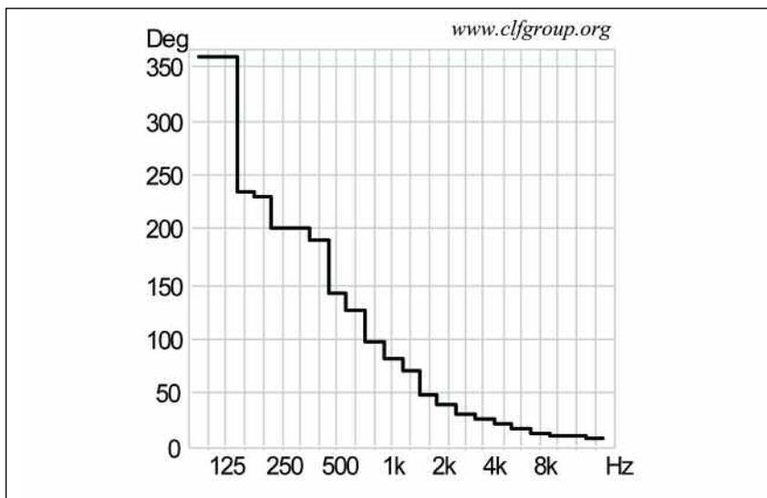
Figure 3 – The vertical beamwidth vs. frequency for a single MiniCOM.P.A.S.S.
