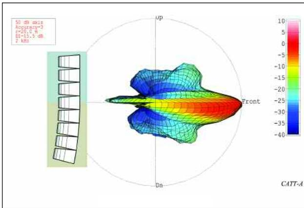
Figure 12 – 2 kHz balloon of Array 2.
