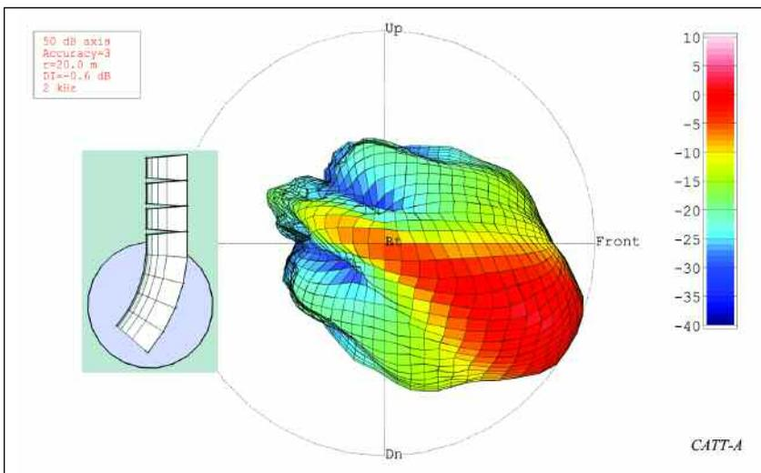
Figure 9 – 2 kHz balloon of the curved segment of Array1.
