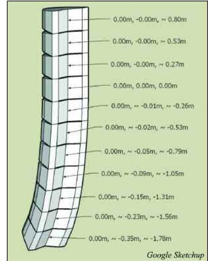
Figure 6 – A Sketchup model gives the box coordinates and angles for CATT-A (Array3 shown).
