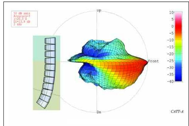
Figure 15 – 2 kHz balloon of Array 3.
