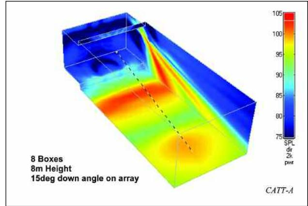
Figure 11 – 2 kHz balloon projected into a room.
