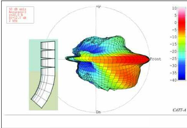
Figure 10 – 2 kHz balloon of Array 1 – all elements on.
