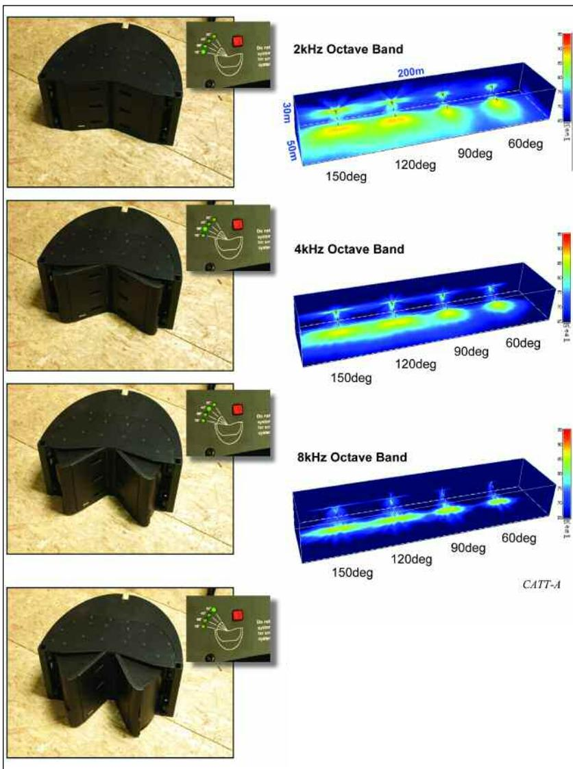
*Figure 5 – Above: Coverage maps of each angle setting modeled side-by-side in a very large room. Note that the actual coverage angle is twice the angle selected on the loudspeaker. CATT-A: Left: The mechanical angle adjustment and corresponding switch setting. There are two switches – one for each sidewall (one shown)*
