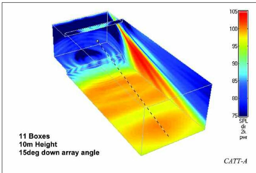
Figure 16 – Array 3 at 10m height.
