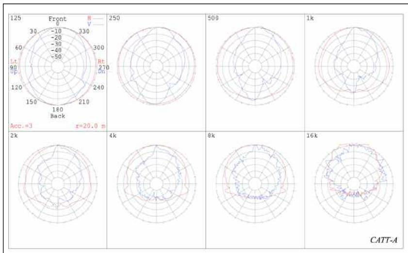
Figure 17 – Octave-centered horizontal and vertical polars of Array 3.
