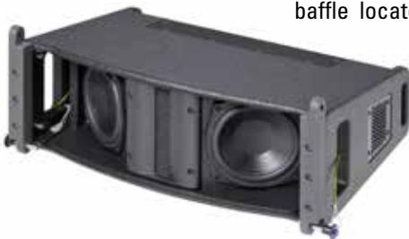
The HF assembly is placed between the woofers: this gives a controlled, symmetrical horizontal dispersion (nominally 100-degrees). The vertical dispersion is sufficiently narrow to
